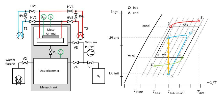
Large Pressure Jump (LPJ), Large Temperature Jump (LTJ), inert-LTJ, and Small Pressure Jumps (SPJ) are "Standard"methods
