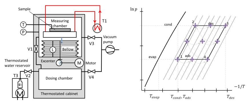
Volume Swing Frequency Response (FR) measurements for in depth investigations of heat and mass as a function of pressure, temperature or loading by model fit [1] in frequency domain.
