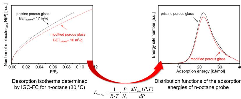
The distribution functions of adsorption energies of n-octane are monomodal, indicating the insufficient character of hydrophobic n-octane as probe molecule for elucidating the surface of hydrophilic silica materials (even after modification by organosilanes).
