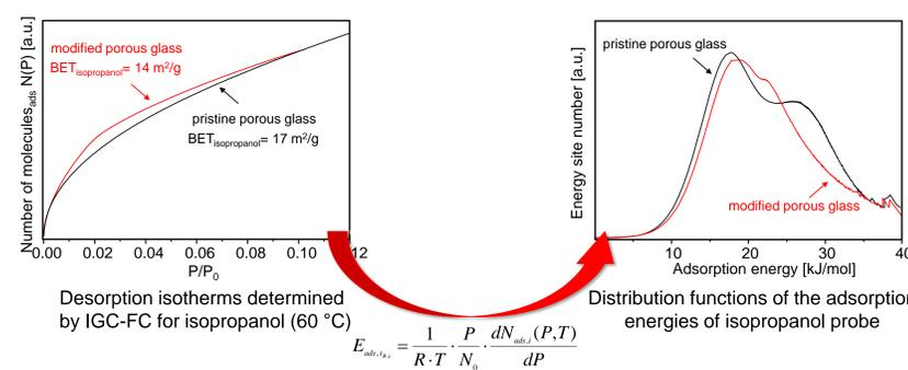
The distribution functions of adsorption energies of isopropanol are bimodal, pointing to the character of the silica surface made of non-hydroxylated (low energy component) and hydroxylated domains (high energy component) which are reduced by silanization.
