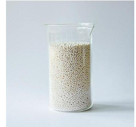
Zeolite for gas purification
