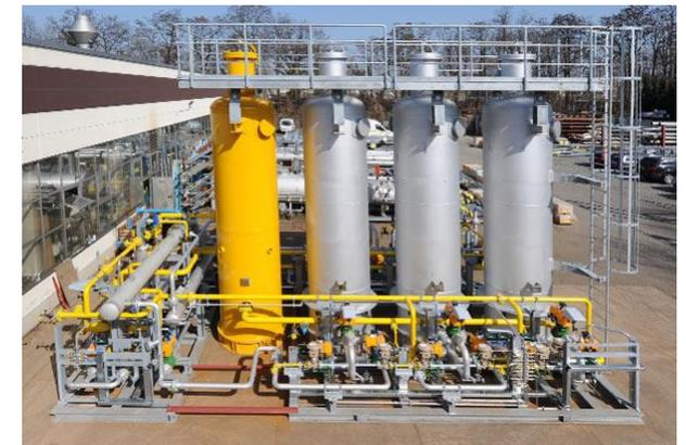
Process gas purification plant
