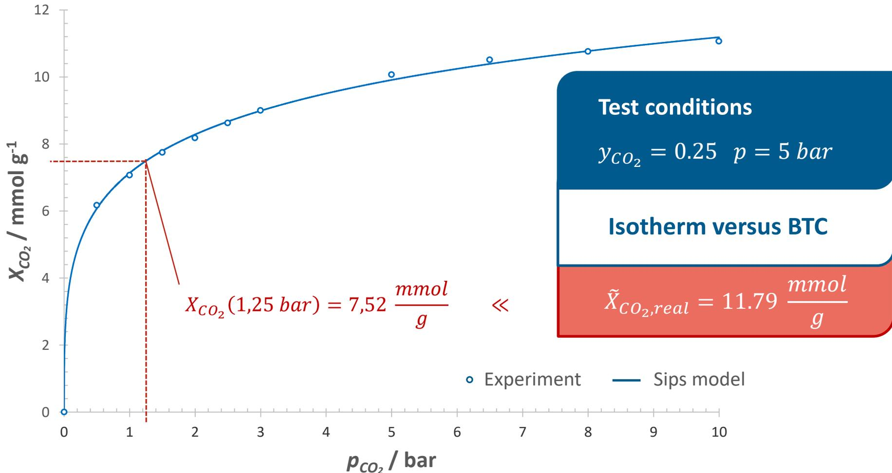
Fig. 6: Adsorption equilibrium of  $CO_2$  on pure NiMOF-74 at  $\vartheta = 30 \text{ }^\circ\text{C}$
