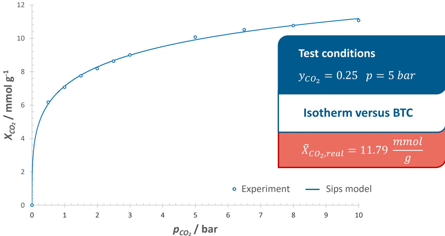
Fig. 6: Adsorption equilibrium of CO<sub>2</sub> on pure NiMOF-74 at  $\vartheta = 30 \text{ }^\circ\text{C}$
