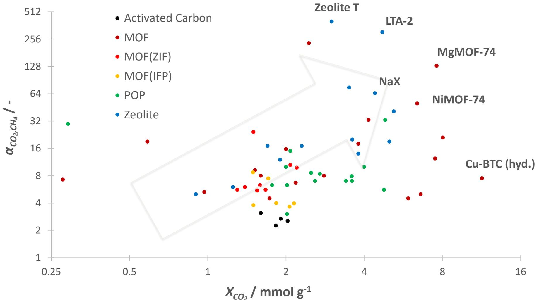
Fig. 1: Equilibrium uptake and selectivity of different adsorbents at STP
