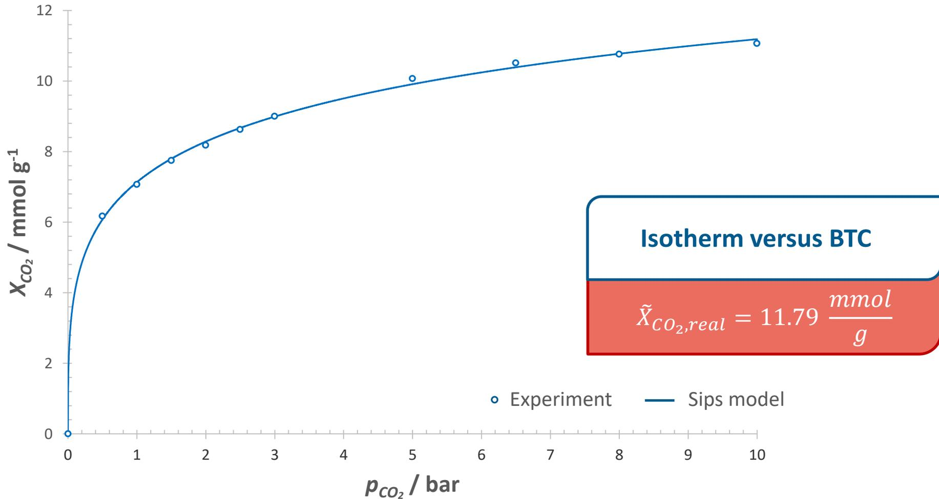
Fig. 6: Adsorption equilibrium of CO<sub>2</sub> on pure NiMOF-74 at  $\vartheta = 30$  °C
