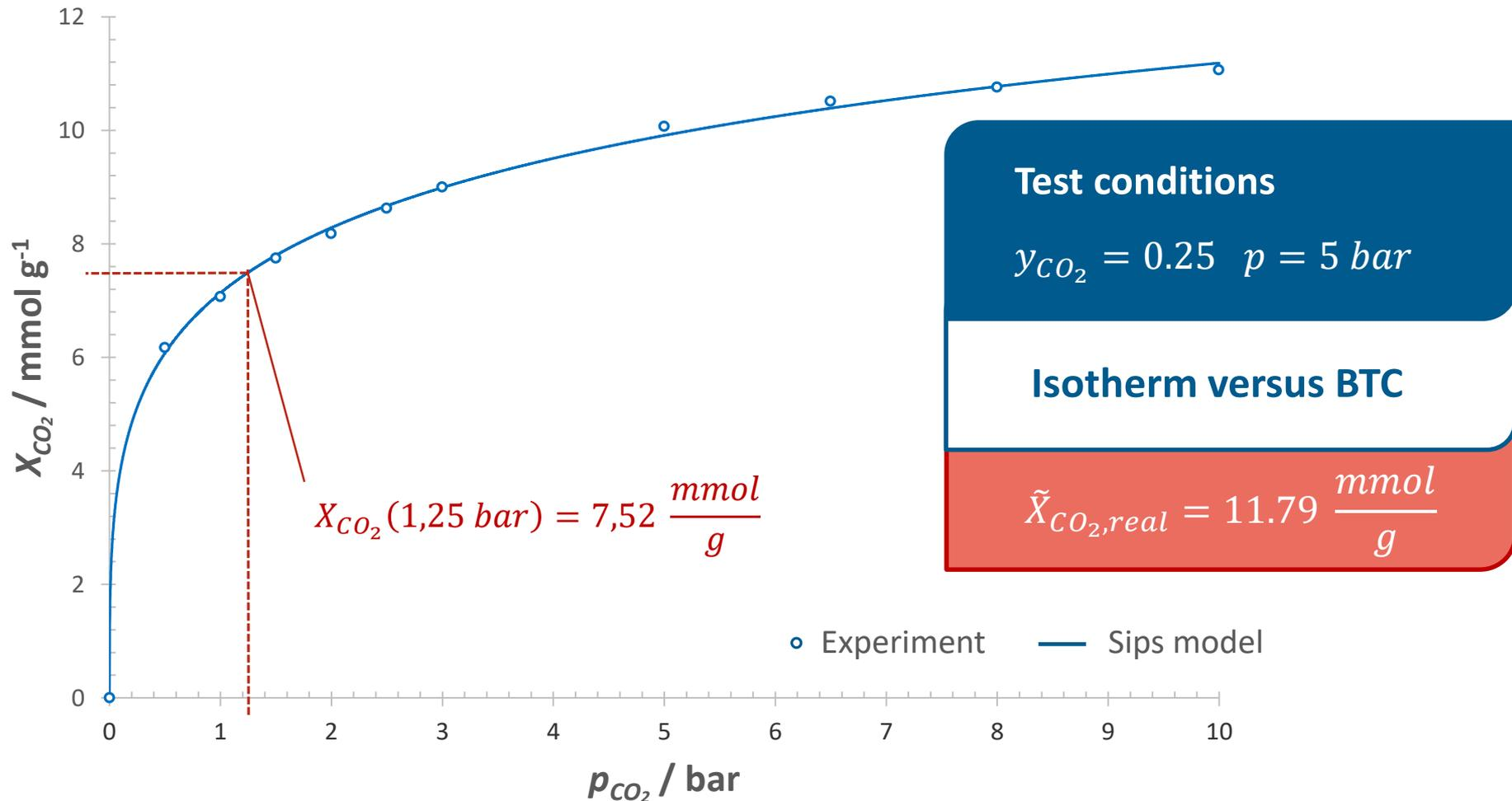
Fig. 6: Adsorption equilibrium of  $CO_2$  on pure NiMOF-74 at  $\vartheta = 30$  °C
