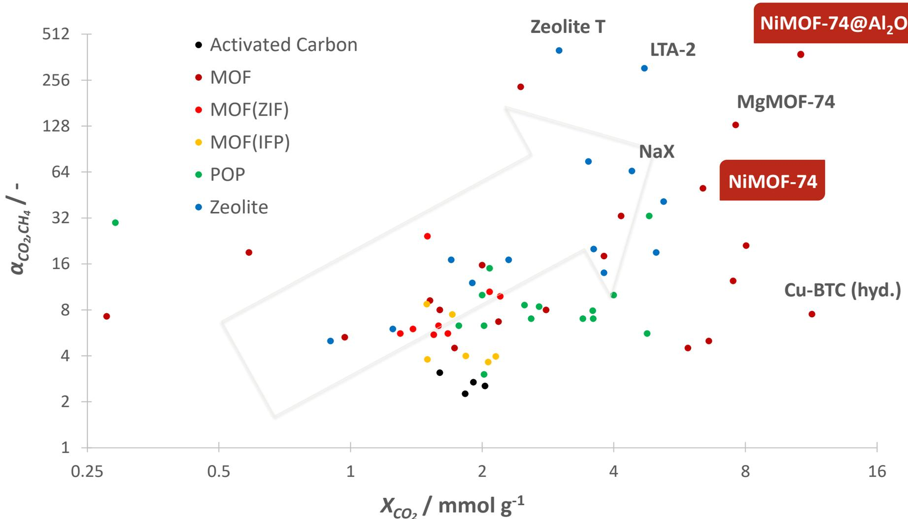
Fig. 1: Equilibrium uptake and selectivity of different adsorbents at STP
